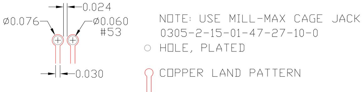
Figure 1. Recommended Geometry for Use with sockets of the CJS01
