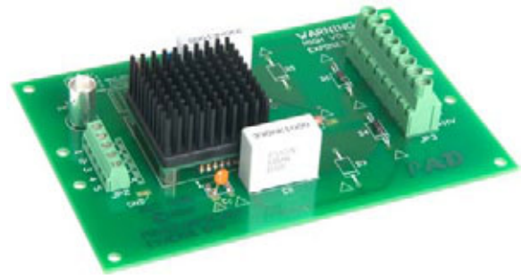
Assembled EVAL195 with amplifier installed.
