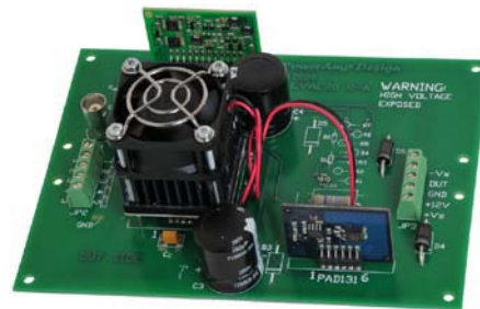
Assembled EVAL20 with PAD20 installed. Optional PAD131 and PAD125 also installed.
