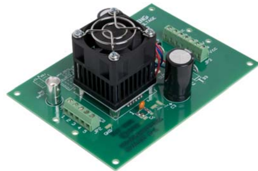
PAD20 INSTALLED IN EVALUATION KIT
